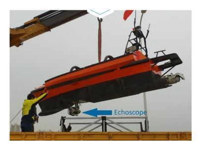
Coda Octopus has recently partnered with AVIC IET, an offshore wind contractor in China, to integrate the Echoscope4G<sup>®</sup> Surface real-time 3D sonar on a state-of-the-art Autonomous Surface Vehicle (ASV).
