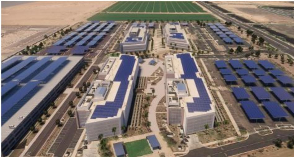
Rendering representative of carport, rooftop and parking garage solar array system designed and to be installed by Ameresco at Wells Fargo's Chandler AZ campus. (Photo: Business Wire)
