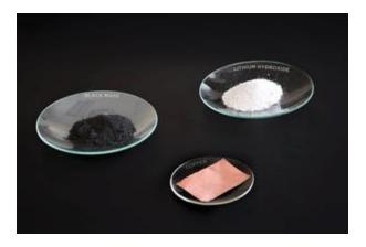
The Copper foil was produced from black mass made up of a mix of lithium-ion batteries. Li AquaRefining will be able to process black mass from any mix of lithium-ion batteries.
