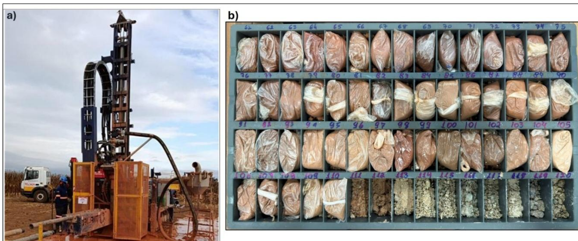
Figure 7: (a) Reverse circulation (RC) drill rig used during the drilling campaign; (b) RC-TGA-0002 drill chip samples showing carbonatite rock chips.
