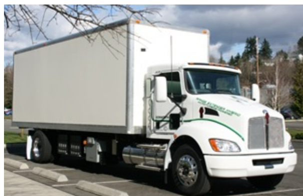
A Capstone C65 microturbine provides extended range by charging a 47kWh Li-Ion battery pack onboard.
