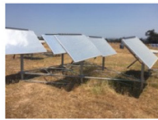
1) Off-the-Shelf Sun-tracking Heliostats (~4 acres per 400 kW)
