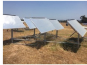
1) Off-the-Shelf Sun-tracking Heliostats (~4 acres per 400 kW)
