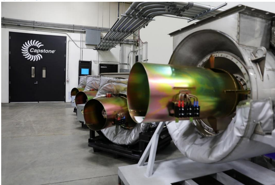
Capstone C200 Engine Source: www.capstoneturbine.com
