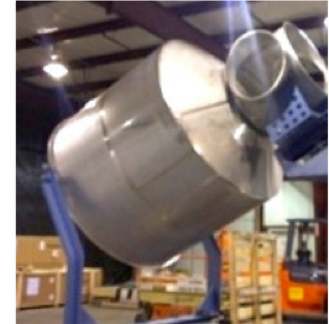
2) Highly Innovative 247Solar Receiver™ (air heating, no moving parts)
