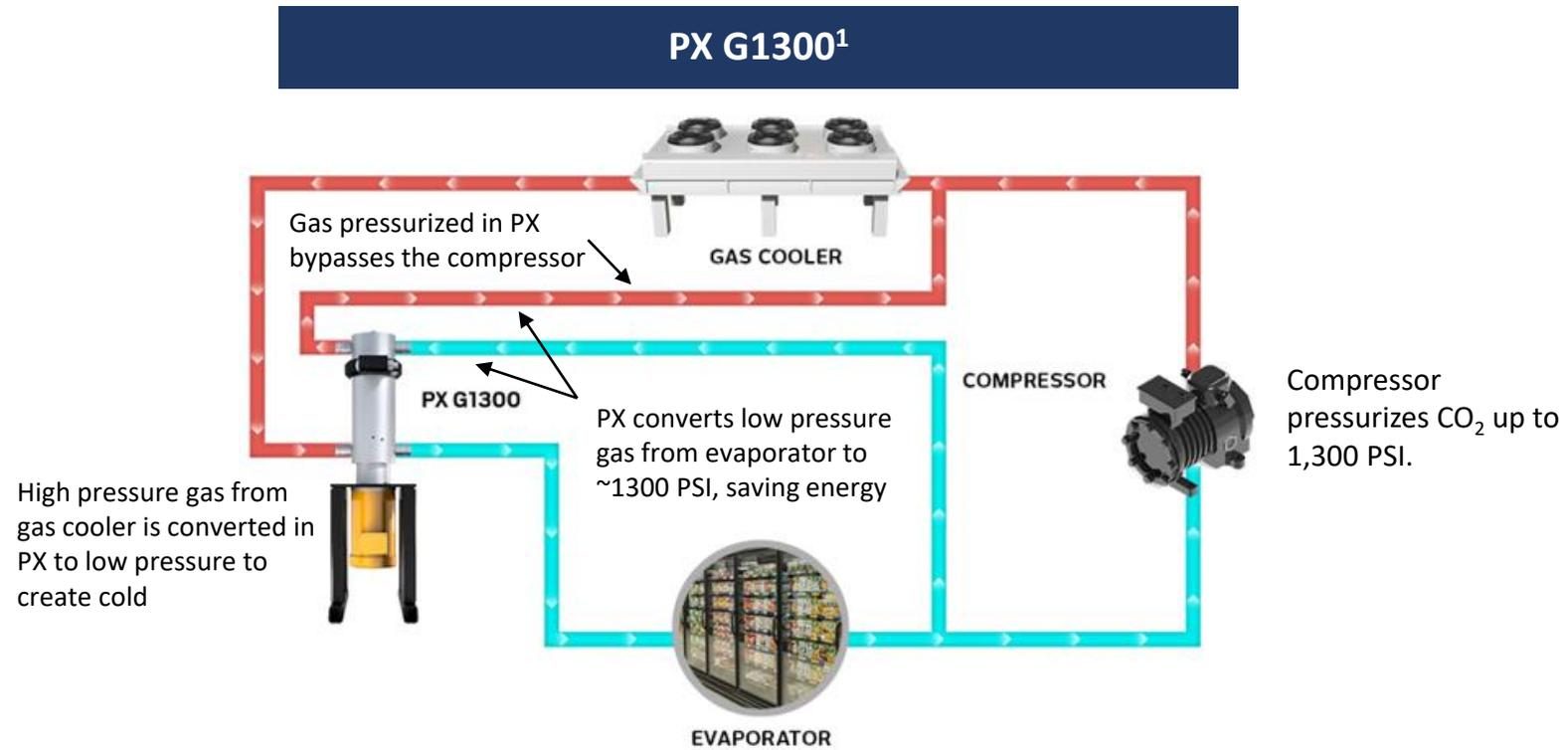
We have expanded the aperture of the PX technology to successfully compress gas, allowing for efficient energy transfer in refrigeration
