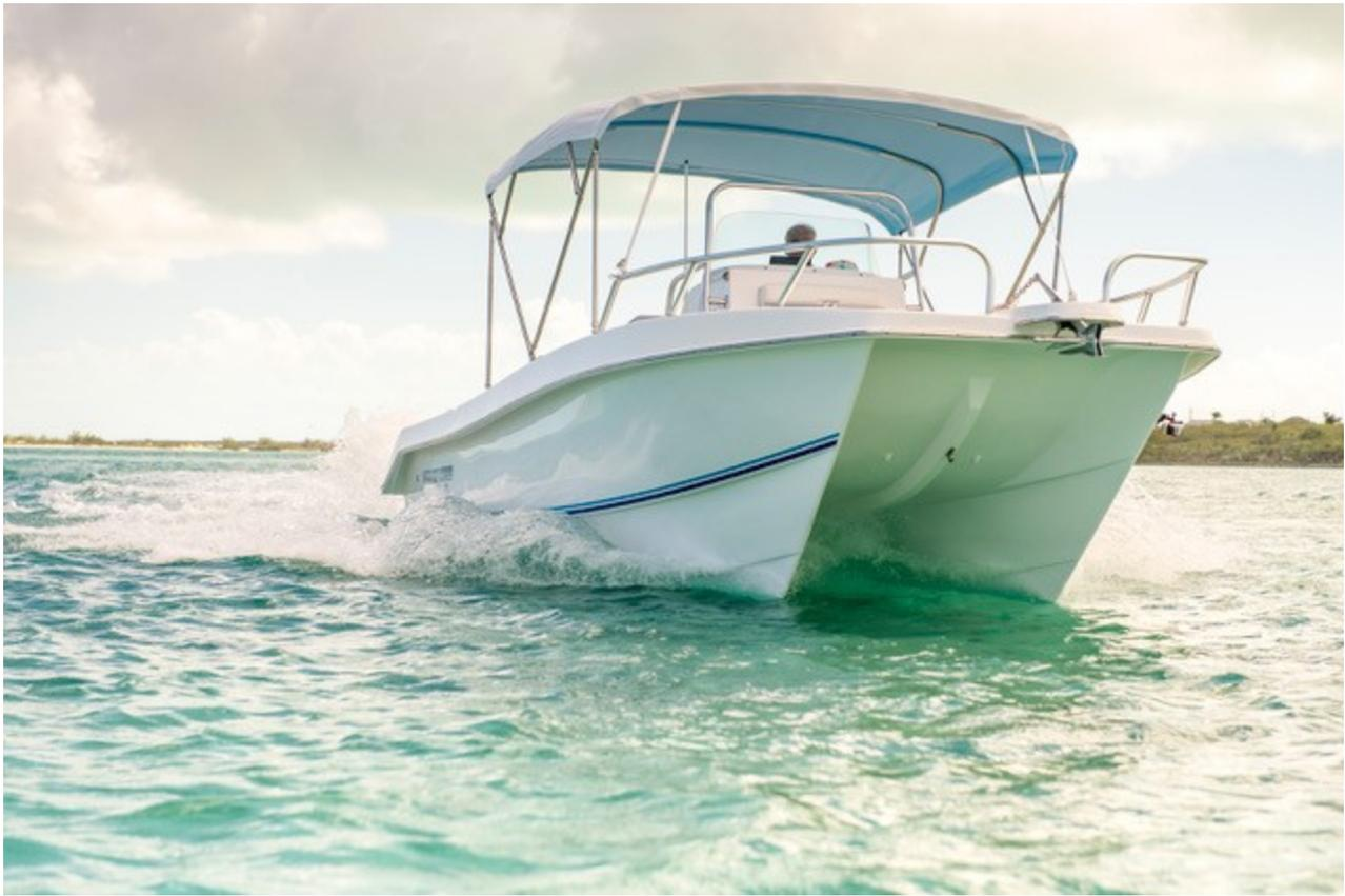
*This Twin Vee catamaran has two hulls, widely spaced, each nearly at her beam ends, rather than a single monohull that is deep on the centerline*
