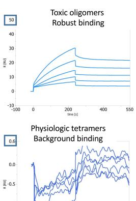
SPR sensorgrams for immobilized antibody and various concentrations of oligomers or tetramers injected over the surface
