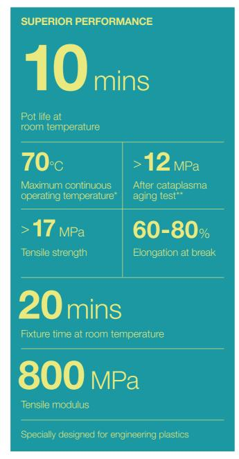
\*For the maximum continuous operating temperature, we consider the maximum temperature forwhich the residual lap shear strength is 1/3 of the lap shear strength at room temperature or the temperature for which the residual lap shear strength is  $\le 5$  MPa. \*\*after 7-days ISO 9142 E2
