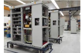
**Level 5:** A fully configured and tested system ready to deliver to the end customer
