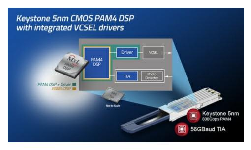
MaxLinear announces 5nm CMOS PAM4 DSP with integrated VCSEL drivers for 800G and 400G Multimode short-reach optical modules and Active Optical Cables (AOC) (Graphic: Business Wire)
