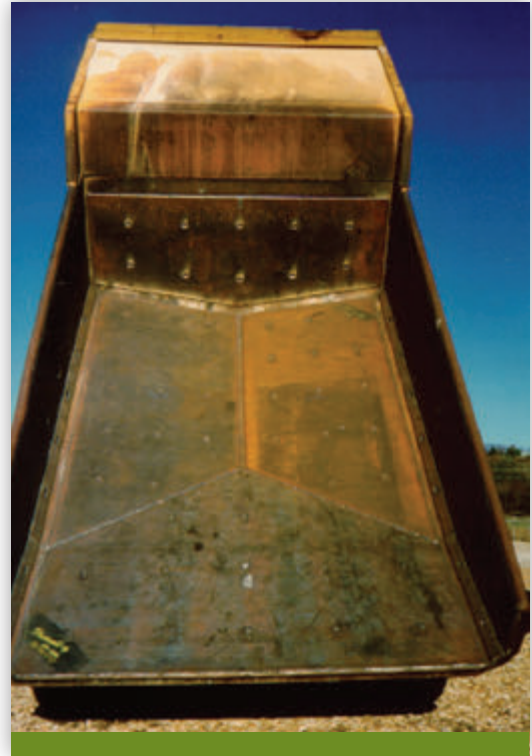
Cleveland-Cliffs' HARDWEAR® steels are used in truck liners. FINELINE™ processing gives them improved toughness and formability.
