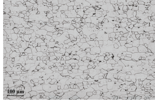
Typical microstructure at 100X original magnification as etched with Vilella's etchant.
