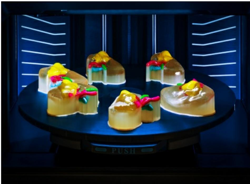
The J5 MediJet 3D printer features a patented rotating build platform with a fixed print head that maximizes reliability and simplifies maintenance. Compared to other 3D printers, the MediJet 3D printer is up to 30 percent faster. (Photo: Business Wire)
