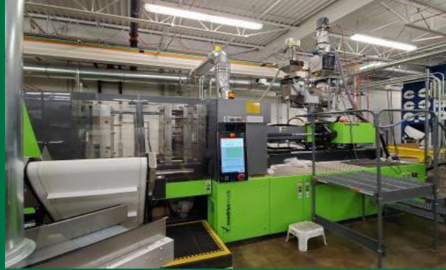
Flea and tick collar injection molding
