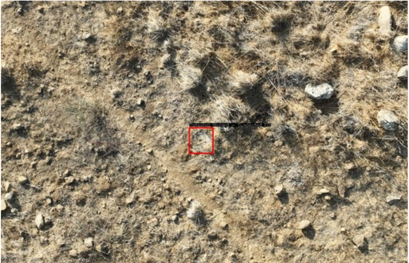
A sample real-world detection of an anti-tank mine identified in drone-based imagery processed by Safe Pro Group's AI platform from a recently completed pilot program conducted in the Middle East (Source: 4M Defense)
