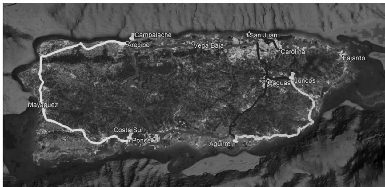
FIGURE 3-2. RECOMMENDED UPGRADE OR RELOCATION OF 230 KV TRANSMISSION LINES
