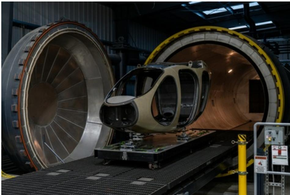
The fuselage of the first aircraft to be produced on Joby's pilot manufacturing line in Marina, CA, heads into a large autoclave to be post cured at a precise temperature and pressure. Credit: Joby Aviation.
