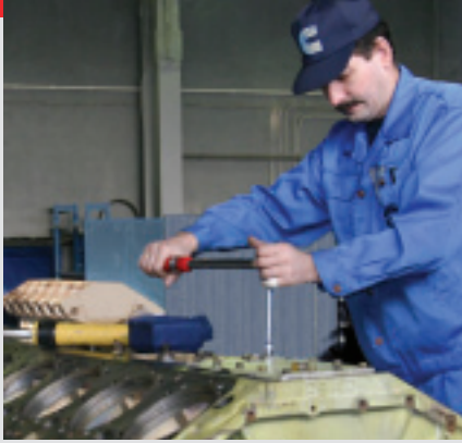
A mechanic in the Cummins distributorship in Russia rebuilds a K2000E engine used primarily in mining applications.
