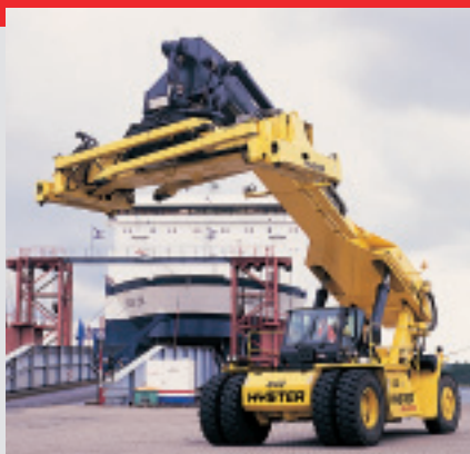
The Hyster reach stacker for container handling is powered by the Cummins QSM heavy-duty engine and operates in ports throughout the world.
