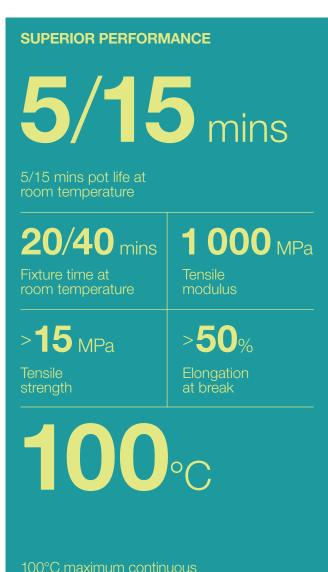
\* For the maximum continuous operating temperature, we consider the maximum temperature for which the residual lap shear strength is 1/3 of the lap shear strength at room temperature or the temperature for which the residual lap shear strength is 5 MPa.
