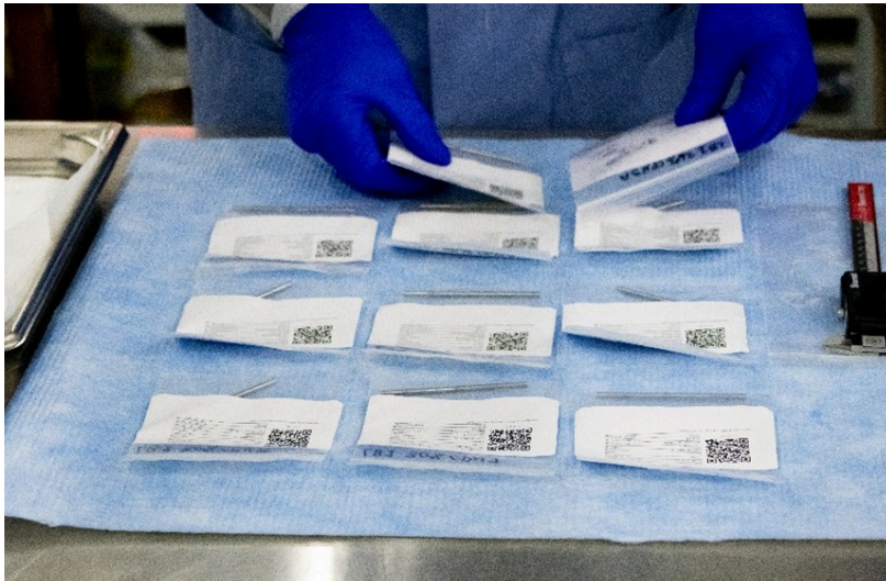
Finished enriched uranium-zirconium coupon samples after characterization and visual inspection results confirmed their suitability for irradiation testing in the Advanced Test Reactor
