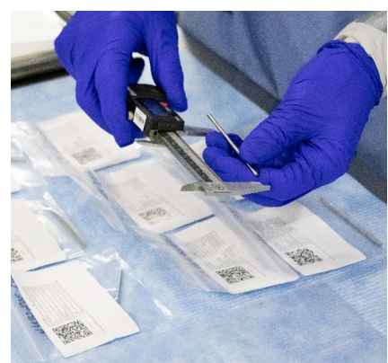
Taking dimensional measurements of a finished enriched uranium-zirconium coupon sample
