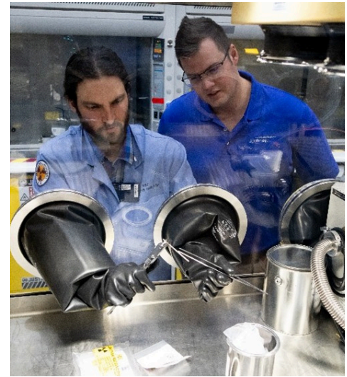
Lightbridge and INL team performing a visual inspection of a finished enriched uranium-zirconium coupon sample inside a glovebox
