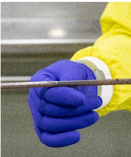
Close-up View of the Enriched Uranium–Zirconium Rod Post-Extrusion, still covered in the extrusion lubricant
