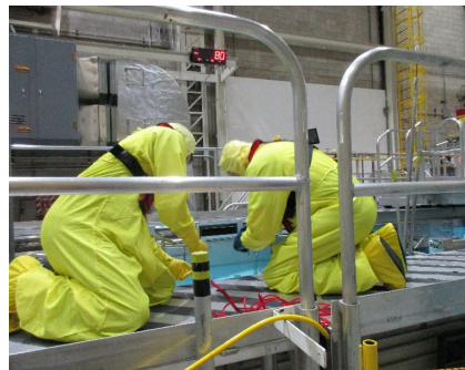
Loading of one of the capsules into an experimental assembly in the ATR canal.
