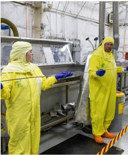
Enriched Uranium–Zirconium Rod Post-Extrusion
