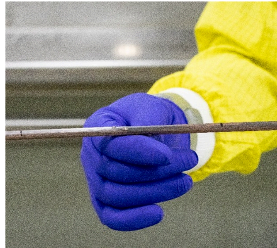
Close-up View of the Enriched Uranium-Zirconium Rod Post-Extrusion, still covered in the extrusion lubricant
