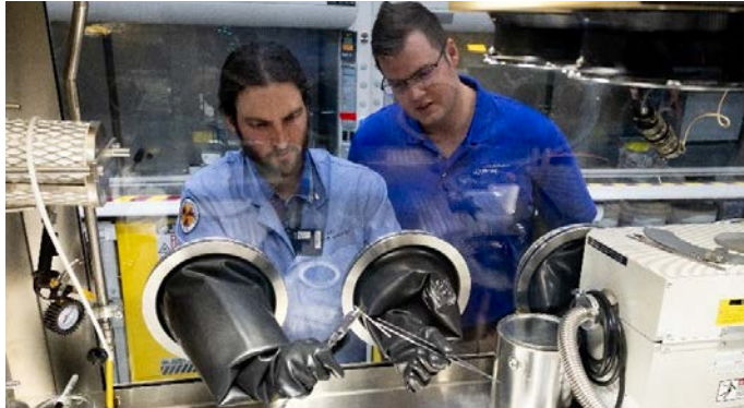
Lightbridge and INL team performing a visual inspection of a finished enriched uranium-zirconium coupon sample inside a glovebox
