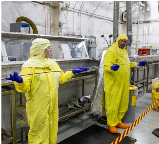
Enriched Uranium-Zirconium Rod Post-Extrusion
