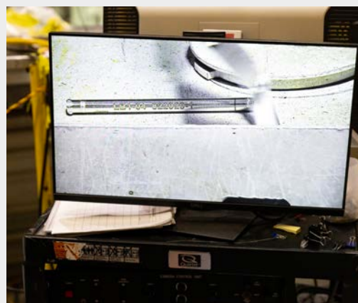
A capsule with an irradiated Lightbridge coupon sample inside after removal from the ATR (May 6, 2026)
