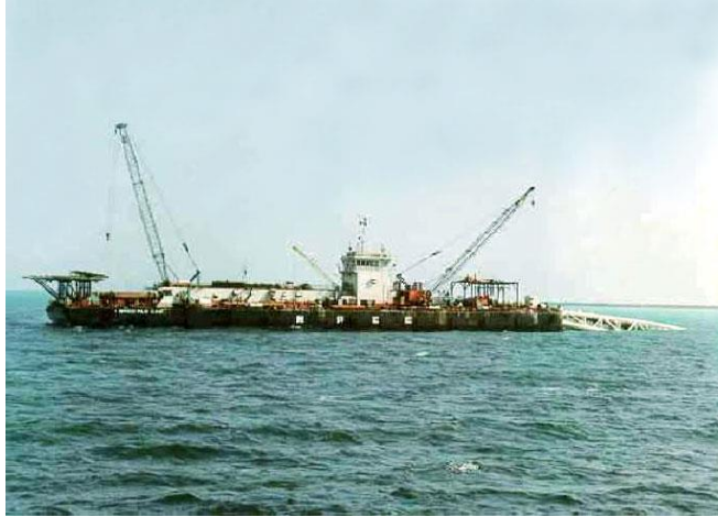
NPCC Pipe Lay Vessel PLB648
