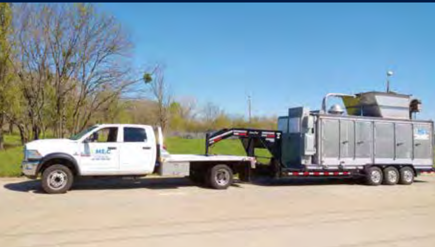
ME 2 C Portable Sorbent Injection System – trailer mounted (above) or stationary (right).
