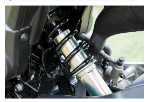
Axalta's Alesta® Spring Black is a new hybrid epoxy powder coating that provides flexibility and mechanical resistance as well as superior corrosion resistance. (Photo: Axalta)
