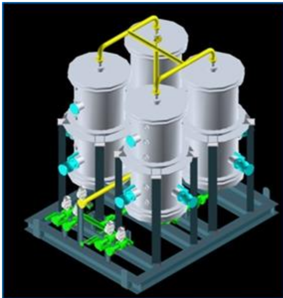
Engineering design of commercial column configuration – SLI's commercial facilities will use the same commercial-scale column, as currently being operated by SLI, in a four pack configuration; the commercial plants are expected to have multiple four packs.
