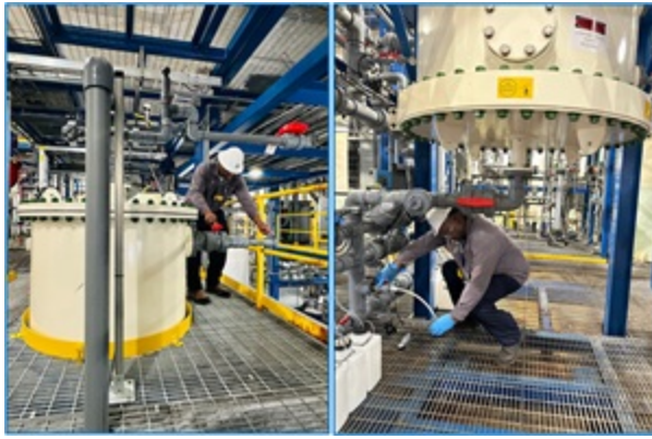
Upper and lower views of the Commercial-scale DLE column in operation at Standard Lithium's Demonstration Plant near El Dorado, Arkansas.
