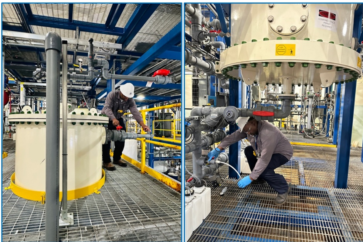
Figure 1 – Upper and lower views of the Commercial-scale DLE column in operation at Standard Lithium's Demonstration Plant near El Dorado, Arkansas.
