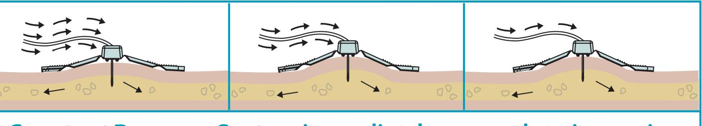
Constant Pressure System immediately responds to increasing pressure in the site(s) by automatically adjusting the flow rate.
