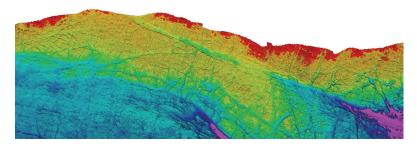
Beautiful rocky coastline off the west coast of Scotland. Data collected using an F185R+™ and an R2Sonic 2024. This data was acquired in very challenging conditions - a sea state 4 with typical swell of 4.0m with up to +-16 degrees of pitch and roll. The extremely accurate performance of the F185R+™ meant no editing of MBES data required. Image courtesy of Aspect Land & Hydrographic Surveys.
