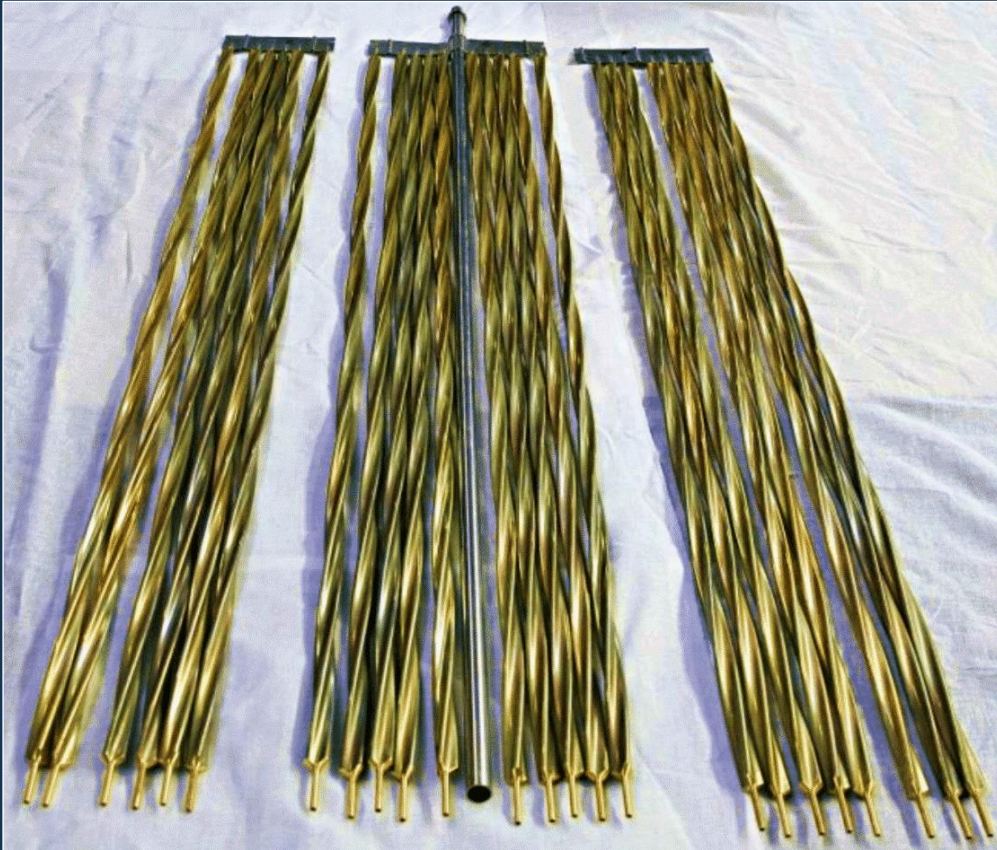
Lightbridge surrogate rods used for a thermal-hydraulic flow experiment
