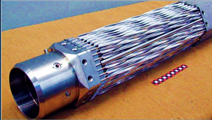
Lightbridge test assembly mockup used for a thermal-hydraulic experiment
