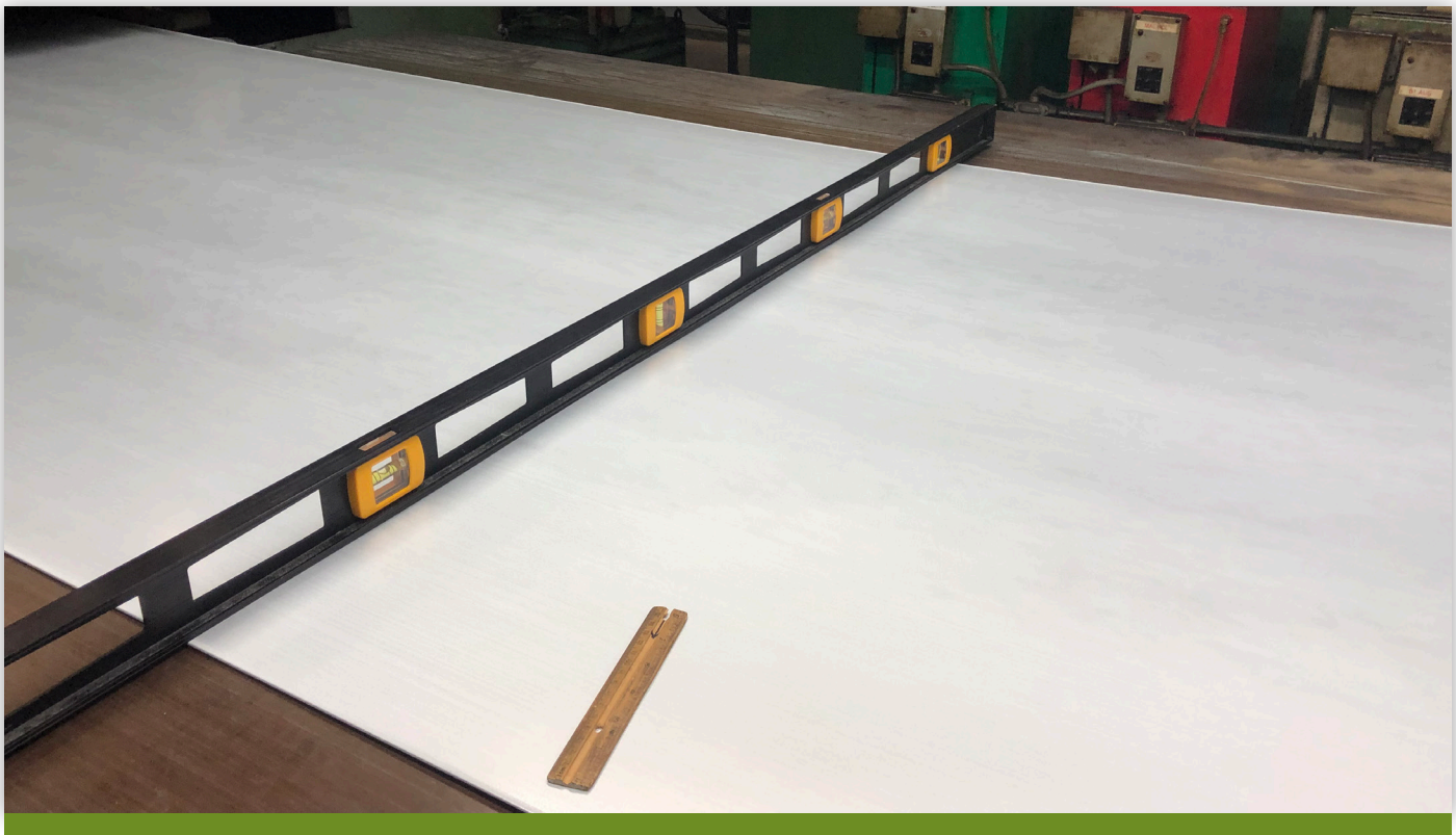
3CAL's world-class flatness. All products produced on the line have comparable shape to that shown in the photo above.
