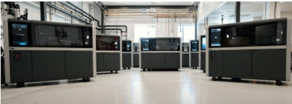
The Desktop Metal Shop System™, the world's first metal binder jetting system designed for machine shops, is being manufactured in volume and shipped to customers around the world. (Photo: Business Wire)
