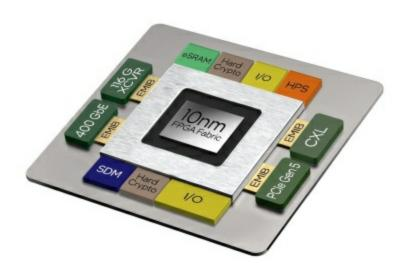
Intel Agilex FPGA family expands with a new FPGA. Agilex 019/023 density devices with integrated cryptography acceleration that can support MACSec in 5G applications. This adds another layer of security to vRAN at the fronthaul, midhaul and backhaul levels. (Credit: Intel Corporation)
