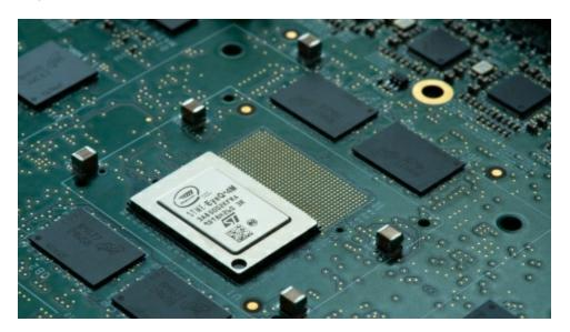
Mobileye's EyeQ4 applies enhanced computational capabilities with computer vision algorithms while rapidly processing information from the vehicle's front-facing camera. With a variety of feature sets including vehicle detection from any angle and next-generation lane detection, the EyeQ4 enables automakers like Toyota to take a major step forward in autonomy, achieving the ability to support and enhance complicated driving tasks. (Credit: Mobileye)
