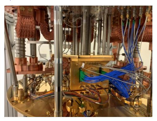
Horse Ridge II, Intel's second-generation cryogenic control chip, brings key control functions for quantum computer operation into the cryogenic refrigerator -- as close as possible to the qubits themselves -- to streamline the complexity of control wiring for quantum systems. (Credit: Intel Corporation)
