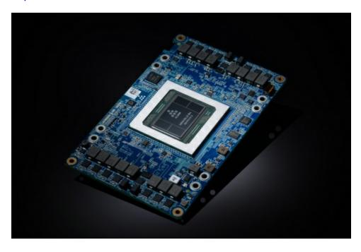
A photo shows Habana Labs' HL-205 Gaudi Mezzanine Card. Gaudi-based EC2 instances deliver cost efficiency and high performance, while natively supporting common frameworks such as TensorFlow and PyTorch. (Credit: Habana Labs)
