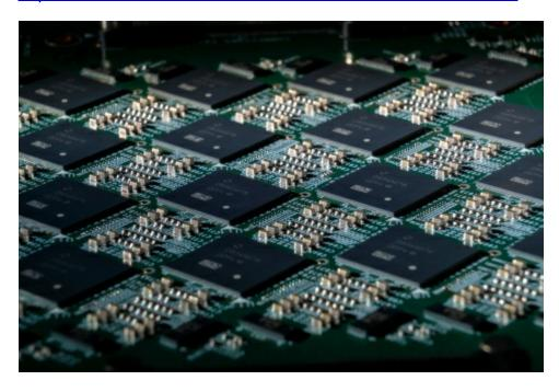
A close-up shows an Intel Nahuku board, each of which contains eight to 32 Intel Loihi neuromorphic research chips. Intel's latest neuromorphic computing system, Pohoiki Springs, was unveiled in March 2020. It is made up of 24 Nahuku boards with 32 chips each, integrating a total of 768 Loihi chips. (Credit: Tim Herman/Intel Corporation)
