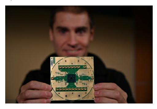
Stefano Pellerano, principal engineer at Intel Labs, holds Horse Ridge. The new cryogenic control chip will speed development of full-stack quantum computing systems, marking a milestone in the development of a commercially viable quantum computer. (Credit: Walden Kirsch/Intel Corporation)
