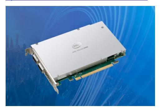
The Intel FPGA Programmable Acceleration Card N3000 is designed for communications service providers to enable 5G next-generation core and virtualized radio access network solutions. Intel Corporation introduced the Intel FPGA PAC N3000 at MWC 2019 in February 2019. (Credit: Intel Corporation)
