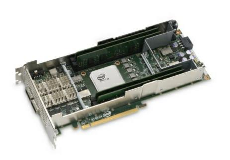
Intel introduced the Intel Programmable Acceleration Card (PAC) with Intel Stratix 10 SX FPGA in September 2018. The card leverages the Acceleration Stack for Intel Xeon CPU with FPGAs, providing data center developers a robust platform to deploy FPGA-based accelerated workloads. (Credit: Intel Corporation)
