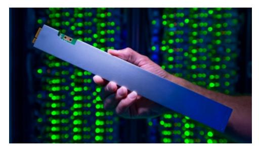
The ruler-shaped Intel SSD DC P4500 can hold up to 32 terabytes. It draws just one-tenth the power of a traditional spinning hard drive. (Credit: Walden Kirsch/Intel Corporation)
