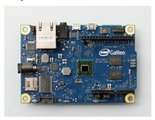
Intel(R) Galileo - Intel(R) Galileo is the first in a line of Arduino-compatible development boards based on Intel architecture. (Photo: Business Wire)
