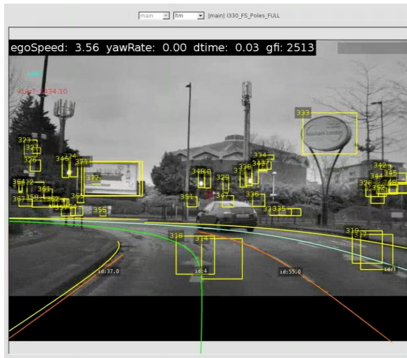
RB data projected onto image space. Road edge, lane marks, lane center, landmarks (in Yellow).
