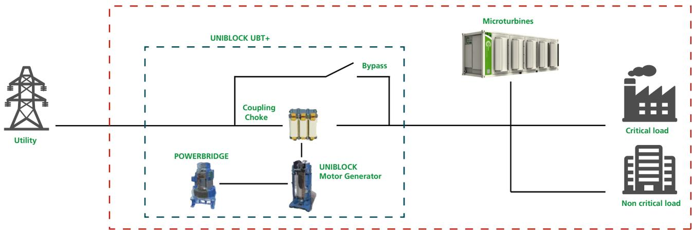
Two Capstone C1000 microturbines operate in concert with a Piller rotating UPS to provide a seamless transition from grid connect operation to island operation.
