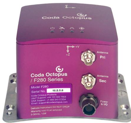
Precision position, heading, heave, pitch and roll in a single compact unit
