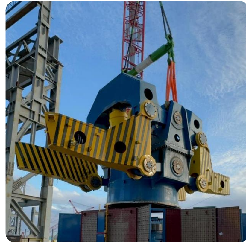
Endless Strip Production caster turret
