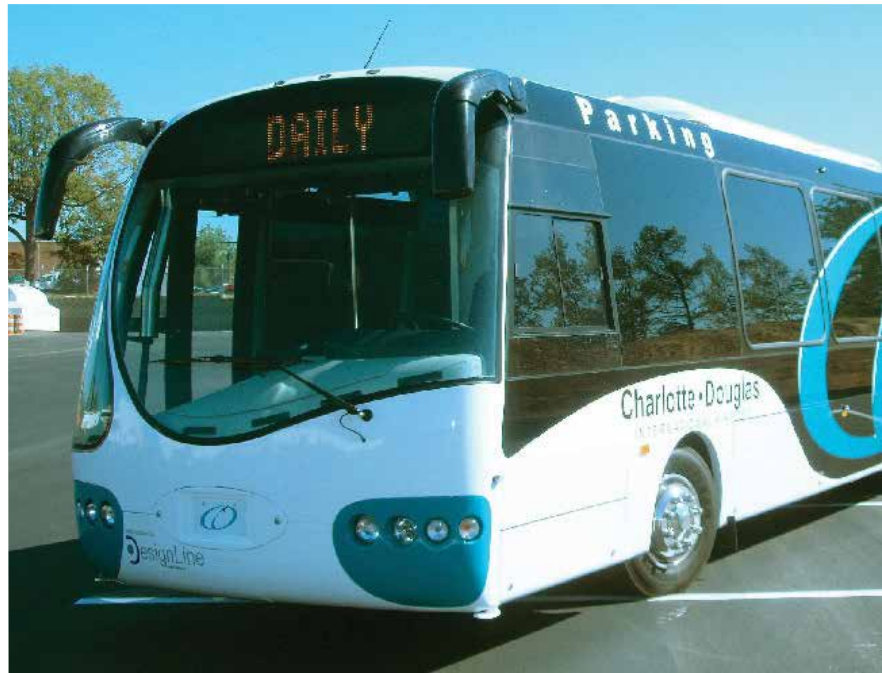
Capstone microturbines generate electricity to charge batteries on HEV buses, even running on jet fuel if needed.
